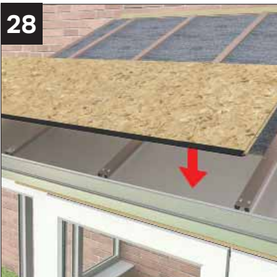
Following location plan, locate first row of OSB panels around the roof using tile starter support section to position. Ensure OSB sheets are the right way up, orientation.
