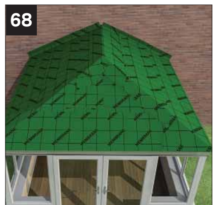
68 Image shows roof covered with breathable membrane. Follow the sequence. Membrane part no: RRMA050
