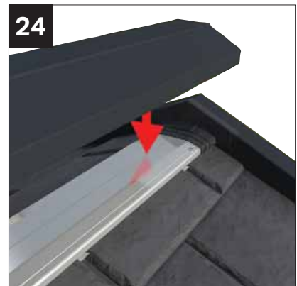
24 Fit the ridge top capping using the NRRSA 005BL supplied.
