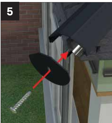
5 Fit hip spine end caps. NOTE: (NRES 004) end cap fixing screw comes complete with 2 part coloured screw cap cover.
