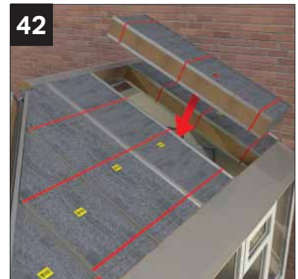
Finally lower into position the expandable panel. Marked with a red label.
