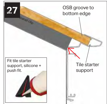
Having silicone sealed the tile starter support onto end of OSB, place tight up to the end of the external panel clip (see red arrow).
