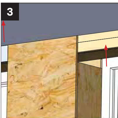
Plasterboard infill to battens adjacent to 12mm OSB cladding.
