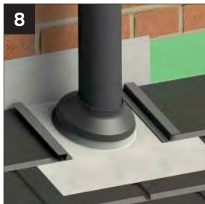
8 A solid roof assembly will look as shown and lead detail comes down the wall directly on to the tiles. Tile cut shown in red.
