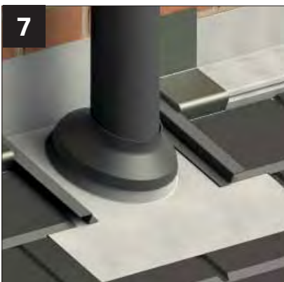
7 Finish with the powder coated rails (supplied) to conceal the cut tile edges before completing the lead detail to finish
