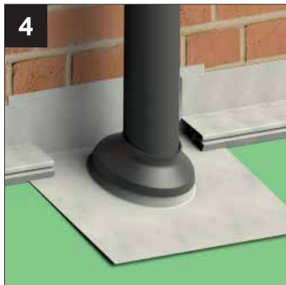
4 Install soil pipe flashing apron (not supplied) over the breather membrane. If your roof features glazing install the tile stop and aluminium flashing cap at this stage at 170mm from pipe centreline.
