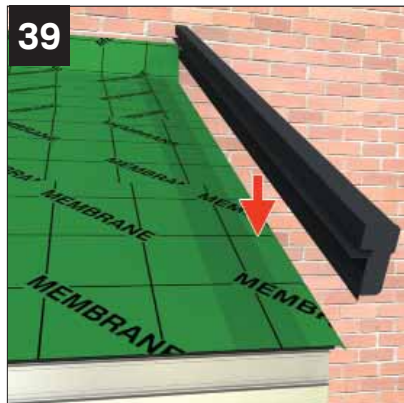
Position the dry verge on the top edge of the bargeboard, with the membrane folded down the face of the barge board.
