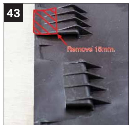
If obstructed on the RHS, remove 15mm from the clips to allow fitting.
