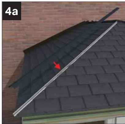
Pre-drill ridge cap at max 750 centres, 6mm holes. 4a Clip fit hip capping, ensure fixing clips are set at 500 centres (pre - fitted clips). In Georgian / Edwardian situation the hip bar cappings are pre - mitred to abut ridge top capping.
