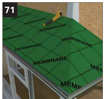
71 Minimum 200mm overlap over hips. Fix using staple hammer with maximum 12mm stainless steel staples. Take care not to cut through lower layers whilst trimming.
