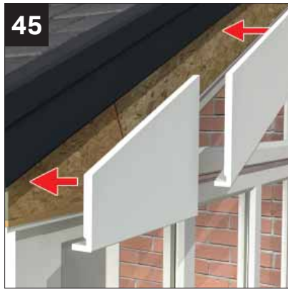
45 Fit pvc barge board box ends and barge board
