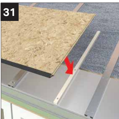
Where required support OSB board at butt joints using timber battens supplied. Battens are 65 x 19 x 700mm long (NRPB010). Only required over box beam.
