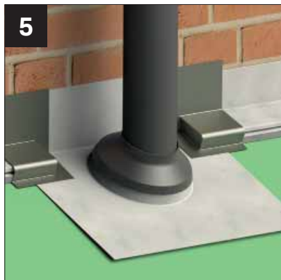
5 If your roof features glazing, flash ends of aluminium flashing caps with butyl patch (supplied) as shown. Cut the patch in half and mould carefully around the contours of the aluminium profiles to form a watertight seal
