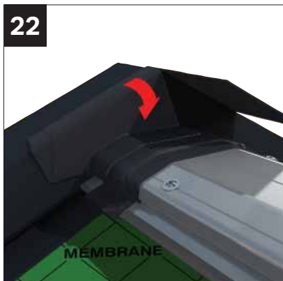
22 Fold down and press firmly into position.
