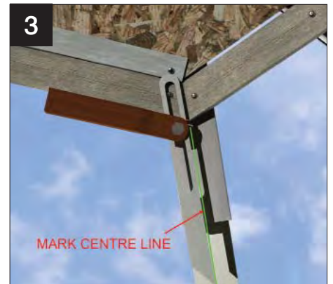
3 Use an angle finder to determine angle of each hip bar.
