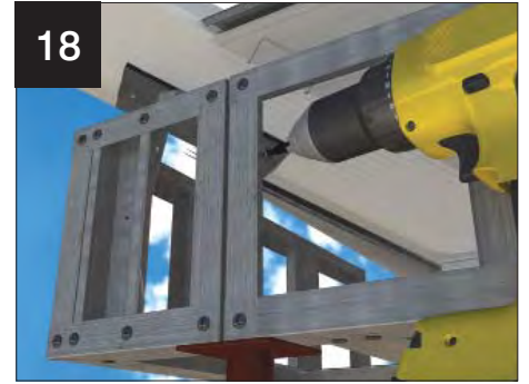
Fit the vertical frames. Fix the frames into the valley corner infill and the horizontal frames.
