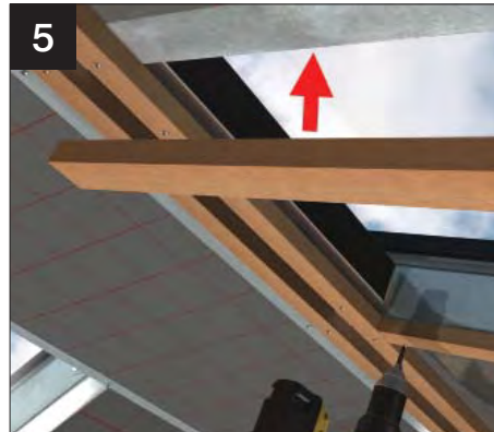
5 Down each side of glazed area, attach batten, ensure it sits 6mm outboard of bolster (see insert).
