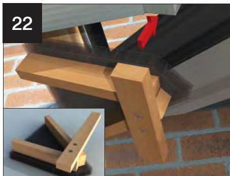
Offer up the cassette assembly into position.
