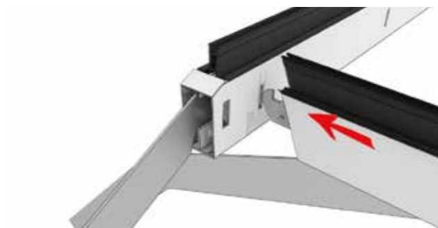
2 Loosen retaining screw from transom connection bracket so that it can move freely and insert transom bracket into slot in the ridge.
