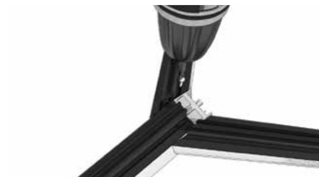
9 Push the joint tight against the ridge and fix down through the rafter with the screw approximately 25mm from the top 4.2 x 25mm screw. Repeat on the opposite side.
